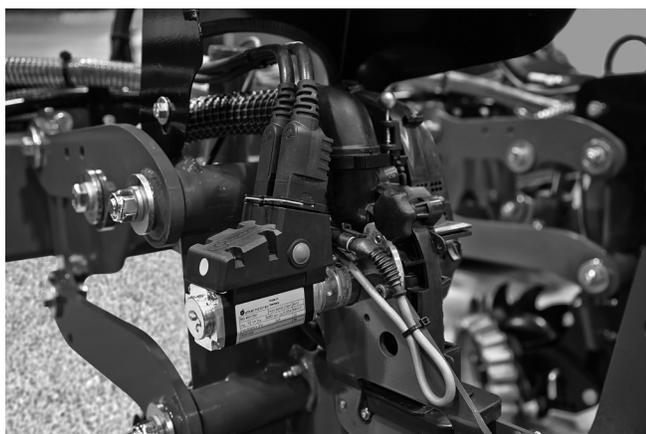
**Figure 4.** Planter row unit with electric seed meter.
